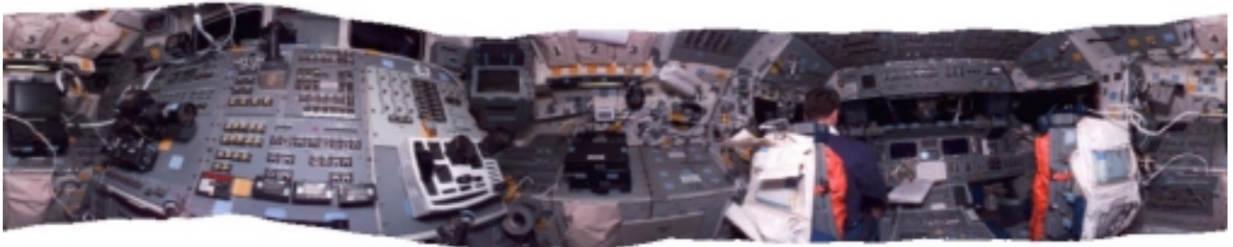
Figure 8: Panorama of Space Shuttle flight deck from 14 images taken with a hand-held camera (using deghosting technique).
